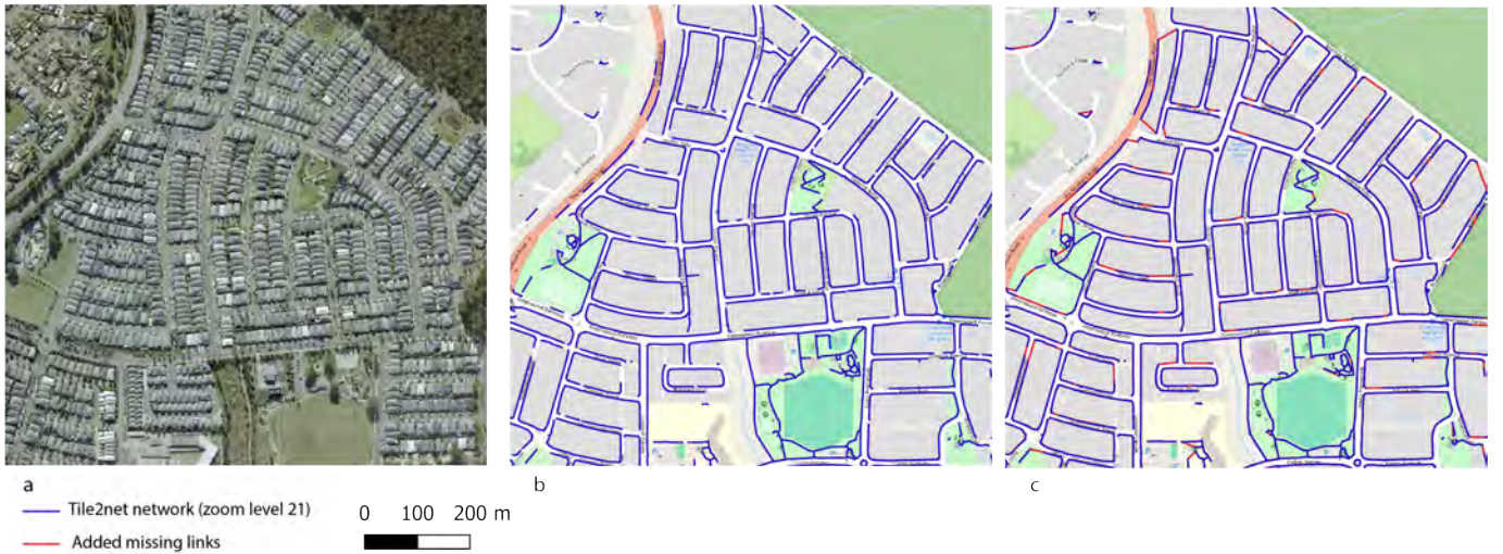
Fig. 1: (a) Aerial shot of Jordan Springs, NSW, highlighting minimal occlusion in the urban landscape. (b) Tile2net Network (c) Resulting network after applying our post-processing heuristic
